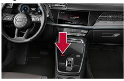
Press the "Start-Engine-Stop" button in the centre console without operating the foot brake.
