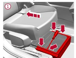
Disconnect the connector on the front of the battery
