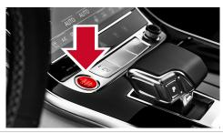
Press the START-STOP button without depressing the brake pedal
