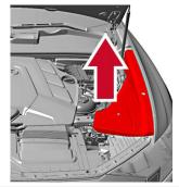
Trigger device that disconnects high voltage
